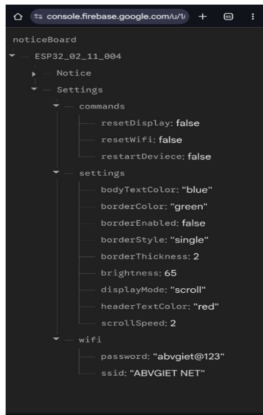
Figure 5.6 Display Configuration Management Interface
